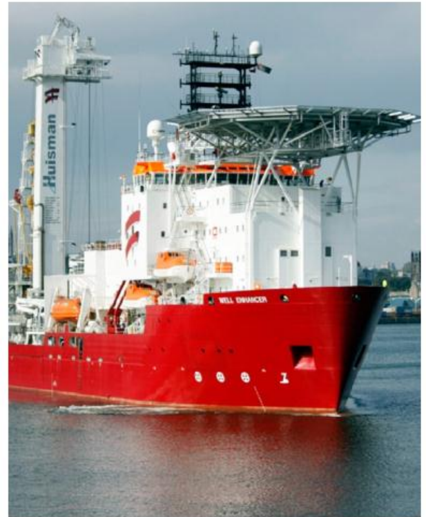
Well Enhancer, operating in the North Sea, is the world's only monohull well intervention vessel capable of deploying coiled tubing
