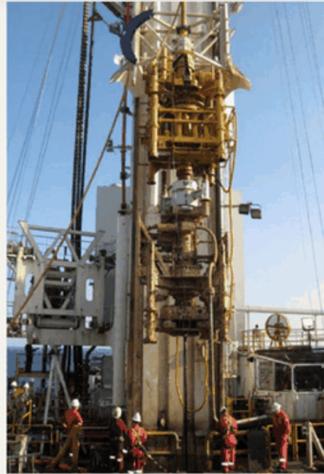
Well Ops' Intervention Riser System recovers a tubing head spool with tubing in one recovery trip
