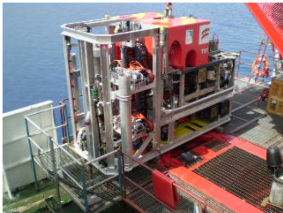
Canyon's ROV Drill Units being deployed on minerals project offshore Papua New Guinea
