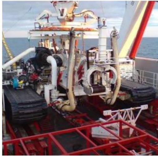
The state of the art I-Trencher system trenches, lays pipe up to 16" in diameter, and backfills in a single operation.
