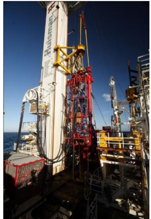
The Compensated Coiled Tubing Lift Frame on the Well Enhancer during its first coiled tubing operation
