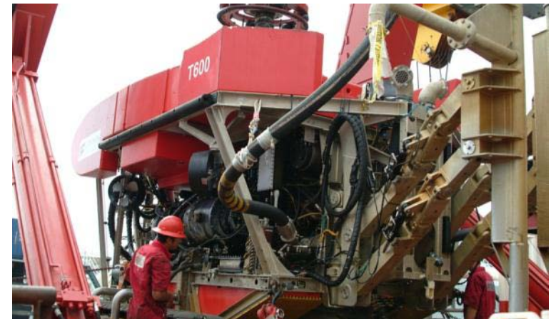
Trenching ROV preparing for deployment
