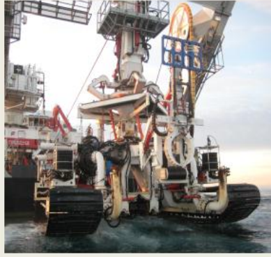
The state of the art iTrencher system trenches, lays pipe up to 16" in diameter, and backfills in a single operation.
