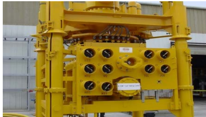
Intervention Riser Systems
