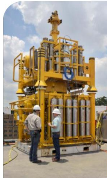
Intervention Riser System undergoing testing
