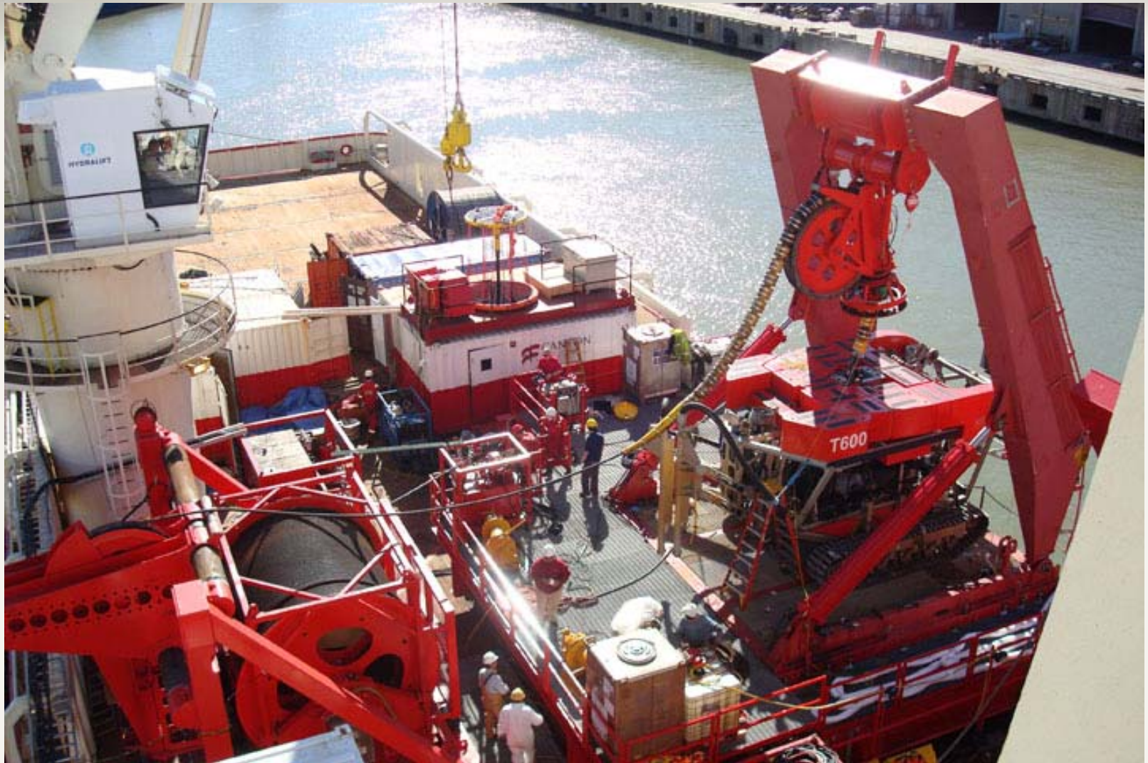
Canyon Offshore ROV spread mobilizing for ENI Pegasus project in the Gulf of Mexico
