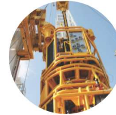
Subsea Intervention Lubricators (North Sea)
