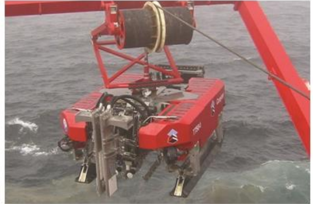
T-750 being deployed for trenching work in the North Sea
