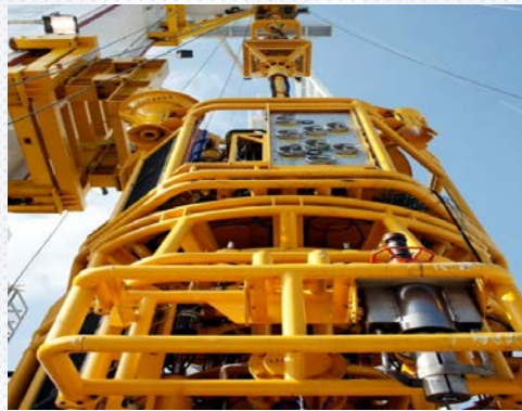
Intervention Riser Systems
