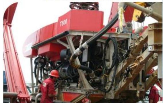
Trenching ROV preparing for deployment
