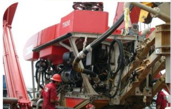
Trenching ROV preparing for deployment
