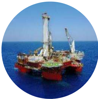
Q4000 (US Gulf Coast / West Africa) Dynamically positioned class 3 ("DP3") purpose-built semisubmersible well intervention vessel
