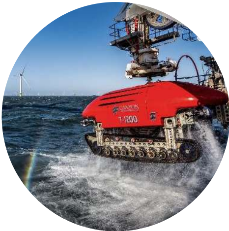
Subsea Trenchers (6 units)
