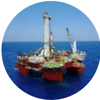
Q4000 (Gulf of Mexico / West Africa) Dynamically positioned class 3 ("DP3") purpose-built semisubmersible well intervention vessel
