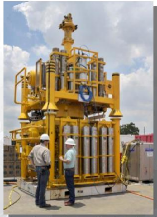
Intervention riser system undergoing testing
