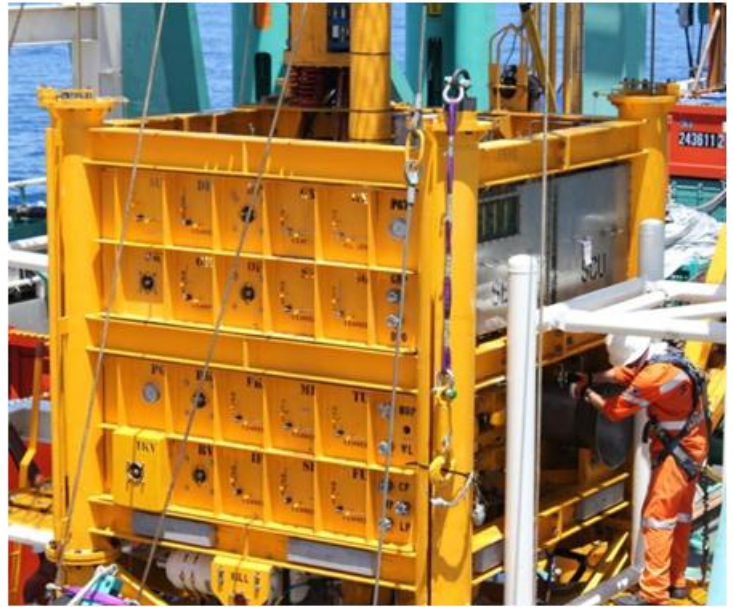
Subsea Intervention Lubricator aboard Normand Clough
