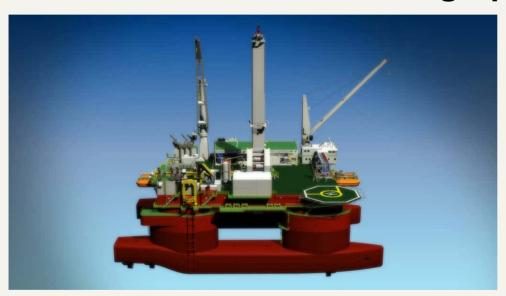
Slimbore drilling capabilities added to a proven rigless well intervention platform ideally suit the Q4000 to meet increasing demand for deepwater drilling services
