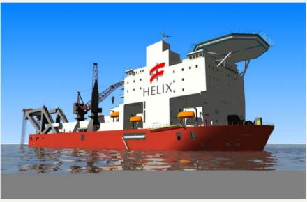
Caesar is among the world's largest deepwater construction vessels, a "floating factory" capable of laying pipelines up to 42 inches in diameter
