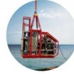
ROVDrill Fully automated seabed operated drilling module capable of carrying out a range of drilling, sampling and in SITU tests
