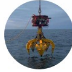
Boulder Grab Remotely operated robotic grab specially developed to relocate seabed boulders to prepare an Offshore Wind Farm site for construction.
