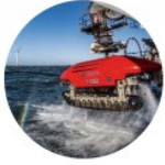
Subsea Trenchers (4 units) Provide subsea power cable, umbilical, pipeline and flowline trenching in water depths up to 3,000 meters
