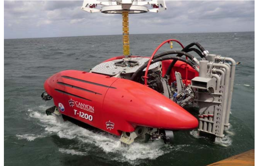
T1200 trencher being deployed
