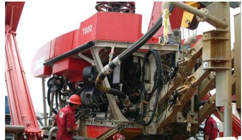
Trenching ROV preparing for deployment
