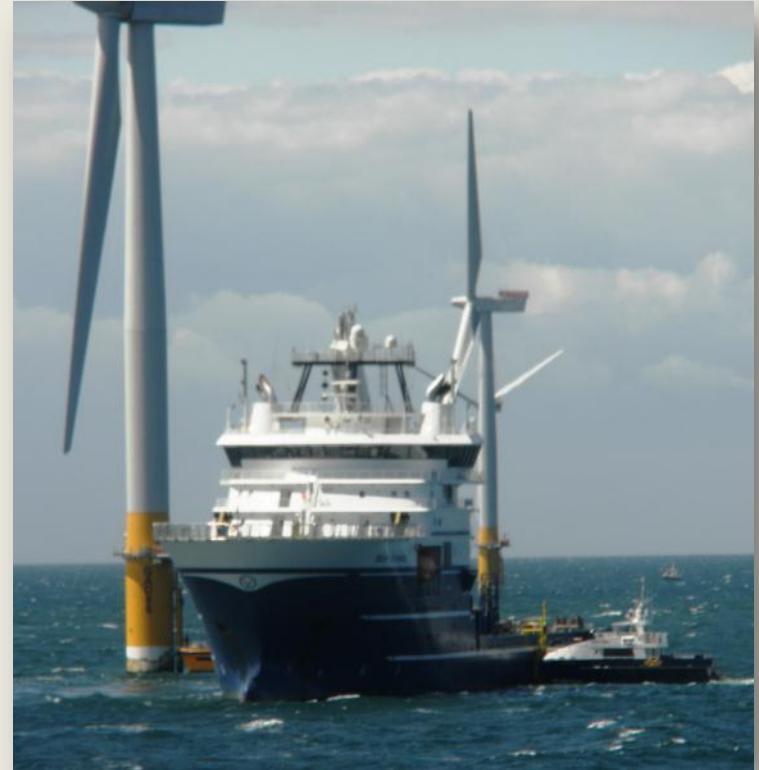
Deep Cygnus performing trenching and cable burial operations at the Greater Gabbard Offshore Wind Farm in the North Sea
