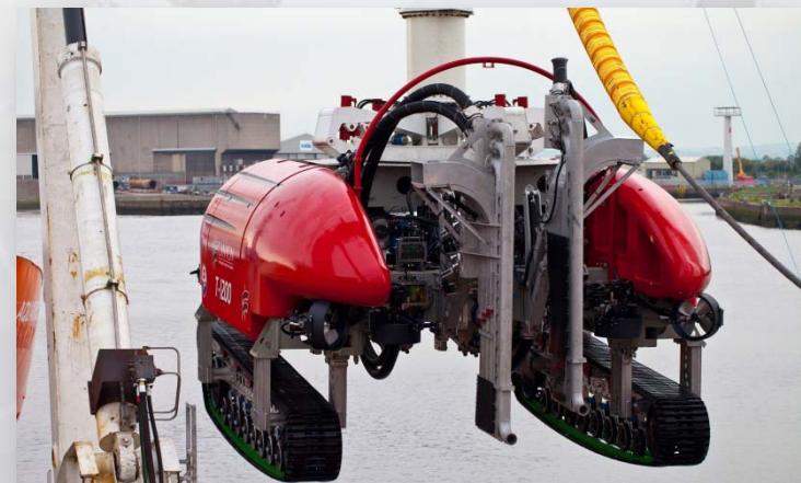
T-1200 Jet Trencher preparing for deployment
