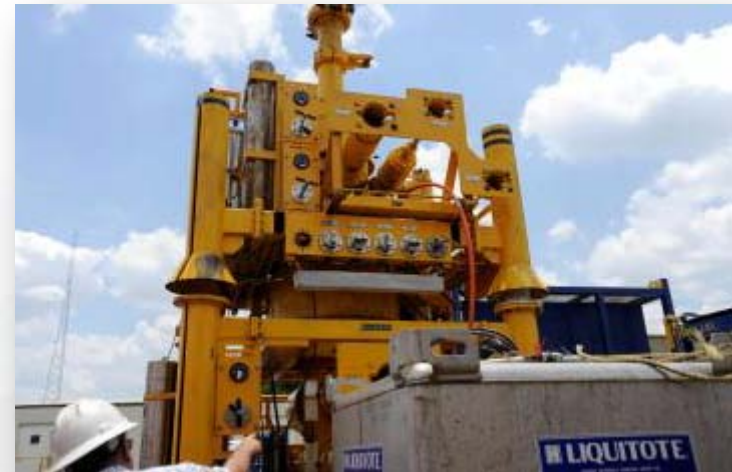
Intervention Riser System
