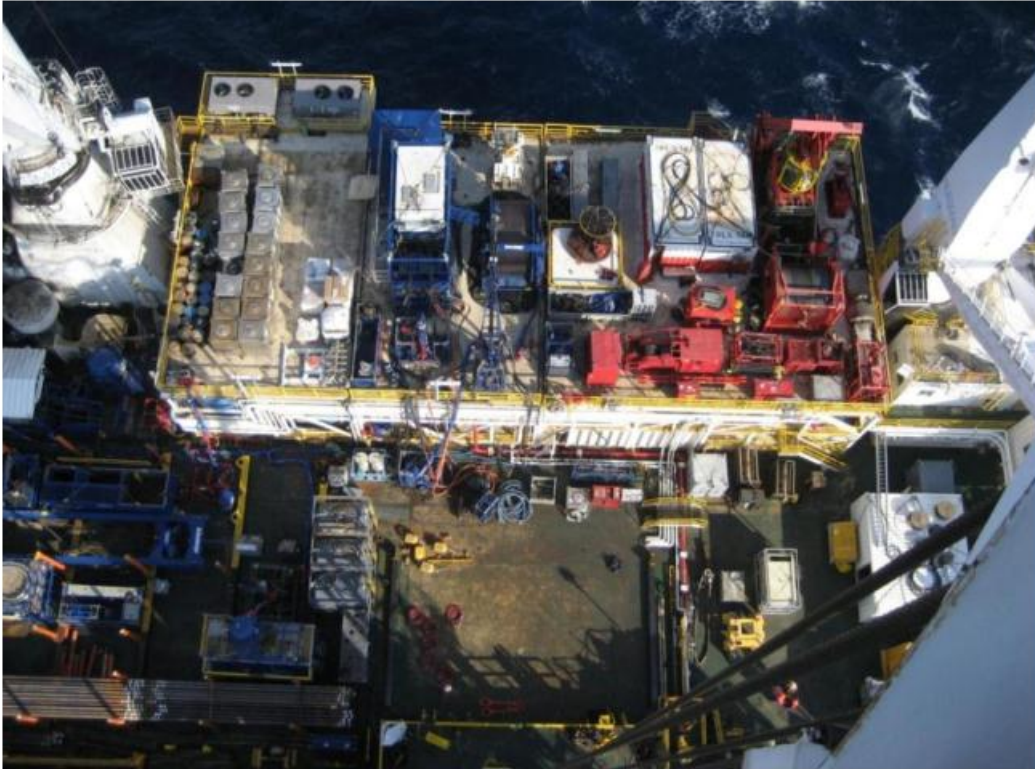
Drilling module roofs with complete coiled tubing system, E-Line, Slick Line, fluids and second WROV system
