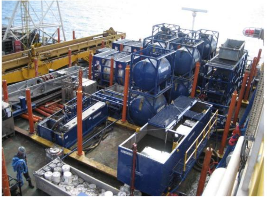
Q4000 Deck Layout for Well Stimulation
