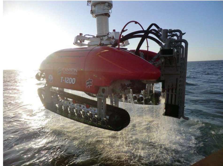
T1200 construction completed, with first trenching job taking place on a North Sea wind farm.
