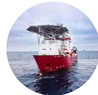
Well Enhancer (North Sea) DP3 custom designed well intervention and saturation diving vessel
