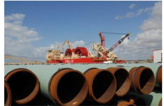
Express spooling pipe in Ingleside
