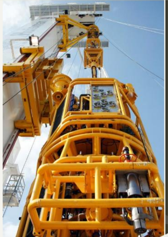
Subsea Intervention Lubricator system onboard Well Enhancer
