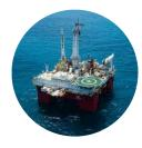
Q7000 (West Africa) DP3 purpose-built semisubmersible vessel for well intervention, decommissioning and other subsea projects
