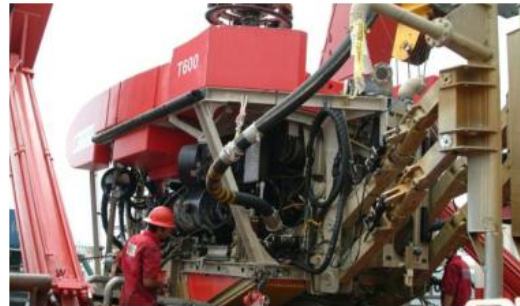
Trenching ROV preparing for deployment
