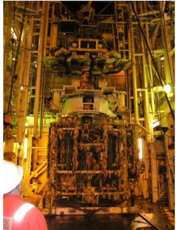
Talisman Xmas tree recovered by Seawell during decommissioning operation
