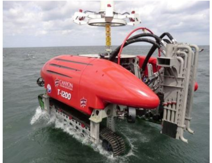
T1200 performs its first trenching operation, burying a 14 km pipeline in the North Sea
