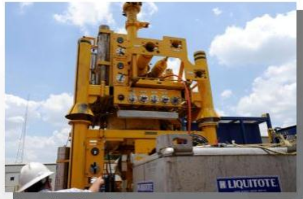
Intervention Riser System
