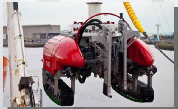
T1200 Jet Trencher preparing for deployment
