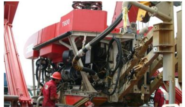
Trenching ROV preparing for deployment
