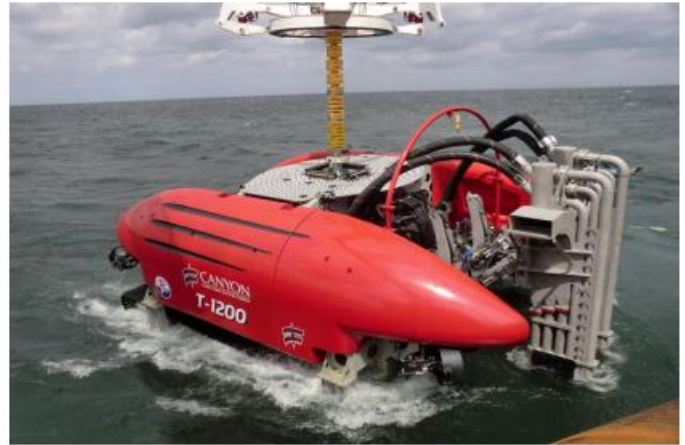
T1200 trencher being deployed
