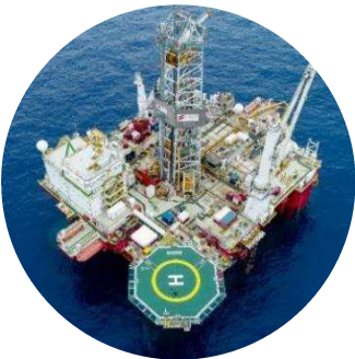
Q5000 (Gulf of Mexico) DP3 purpose-built semisubmersible well intervention vessel
