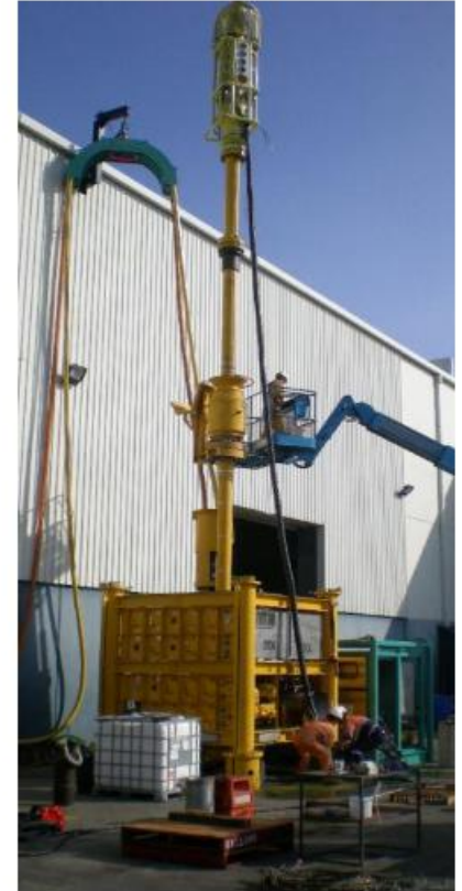
Well Ops APAC Subsea Intervention Lubricator being tested for Well Ops Lufeng project
