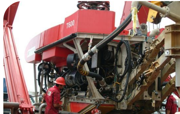
Trenching ROV preparing for deployment
