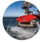
Subsea Trenchers (6 units) Provide subsea power cable, umbilical, pipeline and flowline trenching in water depths up to 3,000 meters
