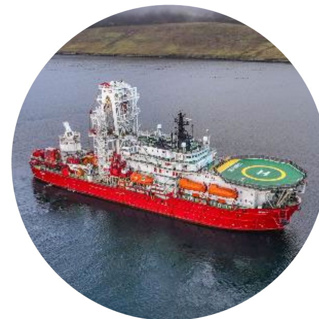
Seawell (North Sea) Dynamically positioned class 2 (“DP2”) light well intervention and saturation diving vessel
